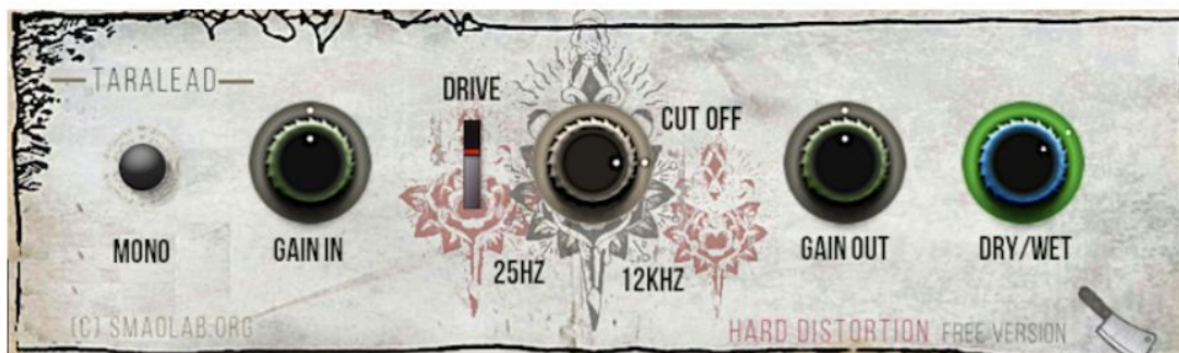
TaraLead – Extreme Distortion plug-in + Asymmetric wave clipping + Oversampling x2
